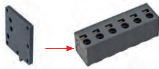
Side Wall with Coding Pin SW-AK4200-CP-V-baGY Article Number: 5420000001 The sidewall with coding pin (SW-CP) ensures the right assembly of the PCB terminal block in the PCB. The coding pin thereby is inserted into the corresponding PCB hole. The SW-CP substitutes the standard side wall (SW).
