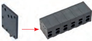
Side Wall with Coding Pin SW-AK4200-CP-H-baGY Article Number: 5420000002 The sidewall with coding pin (SW-CP) ensures the right assembly of the PCB terminal block in the PCB. The coding pin thereby is inserted into the corresponding PCB hole. The SW-CP substitutes the standard side wall (SW).
